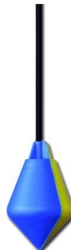
the **level switch** tilts when the liquid level rises in pumping stations, tanks or in any other application where the **float** has been installed. If there is no liquid, the **level switch** remains in a vertical position, suspended by the electrical cable. When the level rises, the microswitch of the **float** will tilt and close or break the circuit. See installations diagrams on the left.
